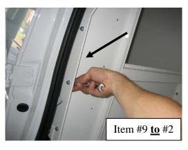
Bolt 3<sup>rd</sup> Compartment Divider to Passenger side Wall using <sup>1</sup>/<sub>4</sub>" x <sup>3</sup>/<sub>4</sub>" carriage bolts, washers and nuts.
